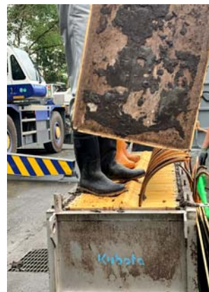
Sludge caking on the membrane plate(element), K-brand
