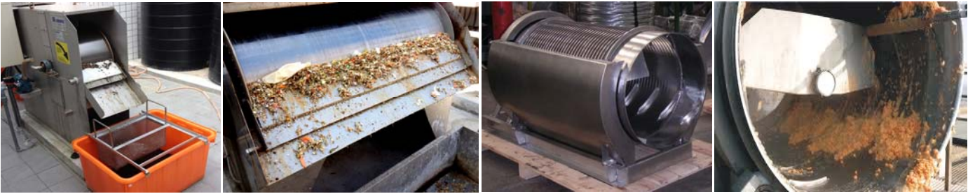
Rotary Drum Screen: External-fed & Internal-fed
