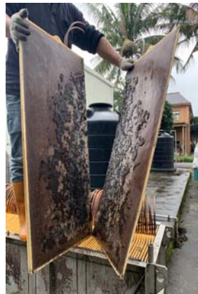
Sludge caking on the membrane plate(element), K-brand
